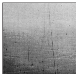
下みがき不十分による研磨キズ Seam and pinhole texture at crossing by less foregoing polish
