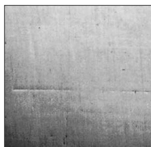
研磨圧力高すぎによる研磨キズ残存 Scratch remains due to overload.
